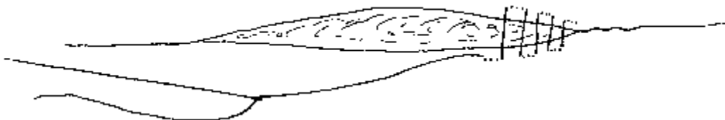
Ladder stitch illustration. The 3 dotted lines represent A stitch under the fabric, not 3 stitches.
